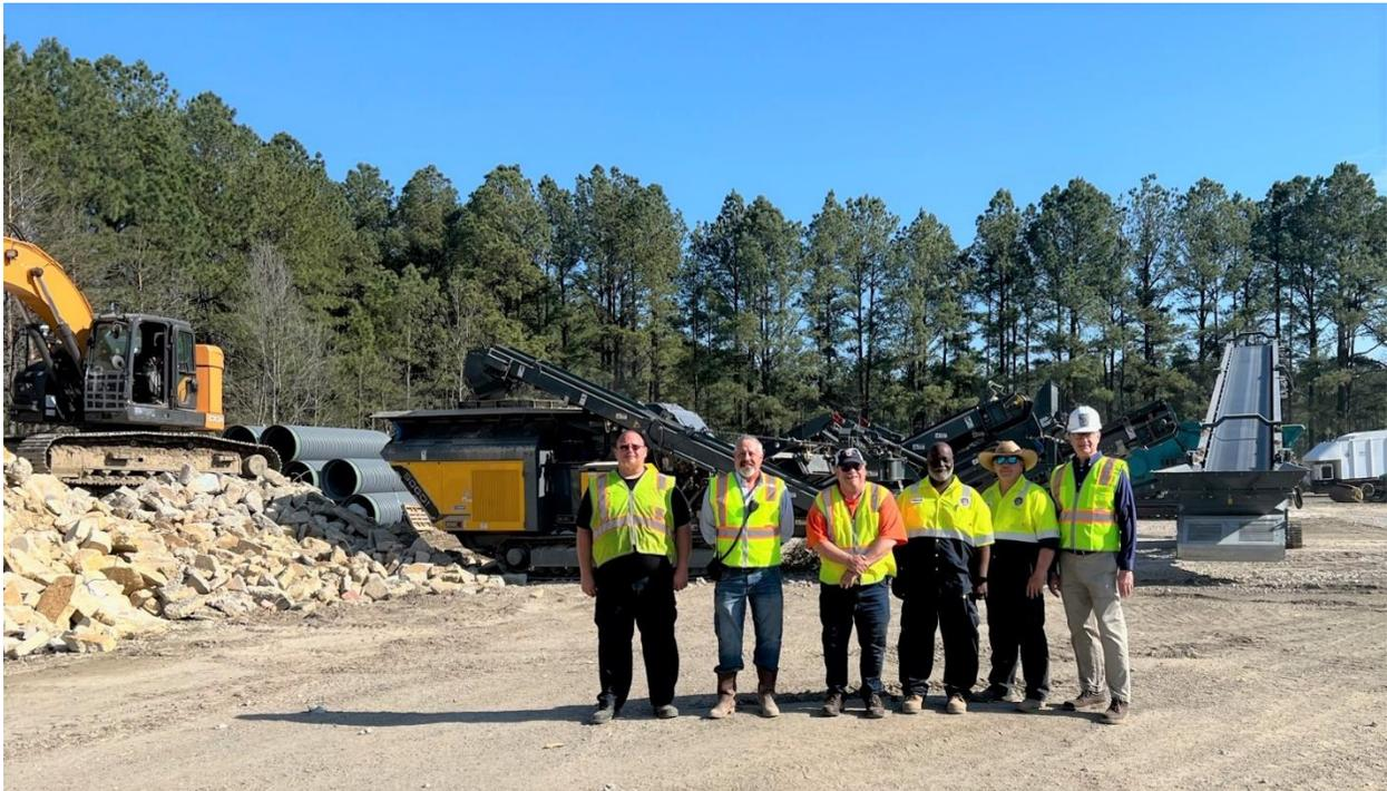
**#2: Pictured are a crusher, a screener, and a trommel at Talbot County's Repurposing Center used to create five recycled materials from both concrete and asphalt.**
